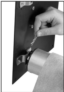
**1)** (For wall mounting only) Remove the small angle-mounting bracket and remount it on the wall side of the plate with the same small bolts.
